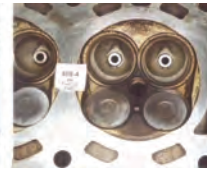
Combustion chamber after P.i. treatment.
