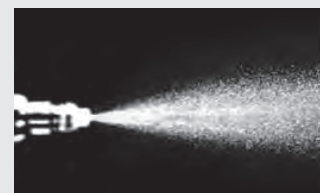
Injector spray pattern after P.i. treatment.
