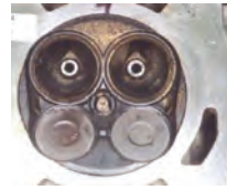
Combustion chamber before P.i. treatment.
