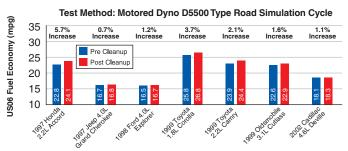
AMSOIL P.i. provided an average fuel efficiency increase of 2.3%, with one car showing improved fuel efficiency of 5.7%.
