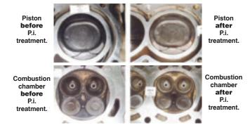
audible knock is controlled, power is lost from retarded timing. Higher octane fuels of 4-5 octane numbers can be used to help prevent knock, an effect called "octane requirement increase." As a vehicle ages, more-expensive, higher-octane fuel is needed to keep it operating at peak performance. By cleaning combustion chamber deposits, knock is controlled, power is restored, fuel economy increases and higher-octane fuels are less necessary for peak performance.
