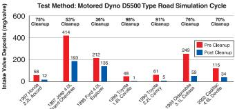
AMSOIL P.i. averaged 72% intake valve deposit cleanup across a wide range of engine types and sizes, with two cars cleaning up greater than 90%.
