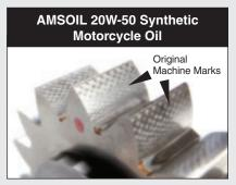
Pass Example: Passed Stage 13, Total Wear, **0mm**
