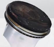
The piston crown contains normal carbon, while the rings remain clean and functional. Note the absence of wear or scuffing on the piston skirt.
