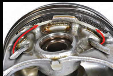
Example of piston damage due to an LSPI event observed during the testing of a competitor's motor oil. The red arrows indicate sections of the ring land that have broken away from the piston.
