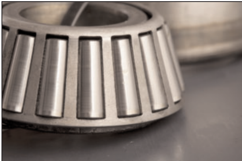
Pinion tapered roller bearing in like-new condition.
