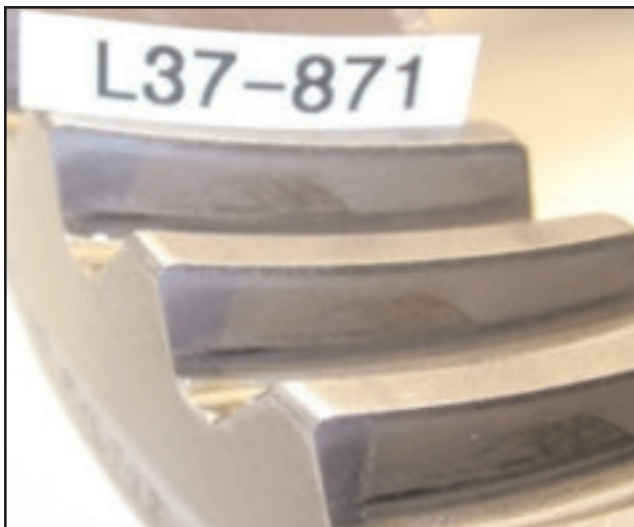
Ring gear exhibits very low wear.
