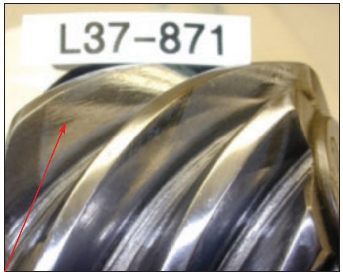
Pinion gear - original machine marks still present.
